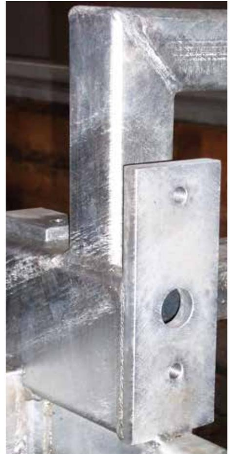
Machined Mounting Pads/Tubular Steel Frame
