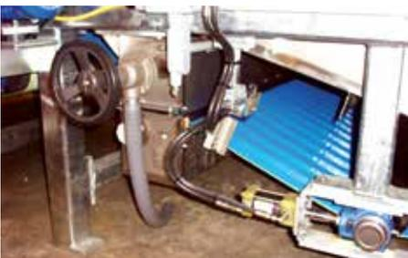
**7 Tubular Steel Frame:** Significantly easier to keep clean. Extremely high moment of inertia (bending and radial inertia 3 to 10 times that of competitors') Hot dipped galvanized inside and out. Precision machined bearing and cross member mounting pads for accurate bearing, roll and frame alignment.
