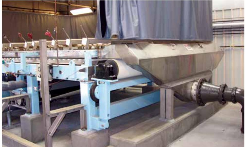
**Venturi Mixer:** Provides excellent dispersion of flocculent. The adjustable counter-weighted baffle allows efficient optimization of slurry flocculation for shortened drainage time.
