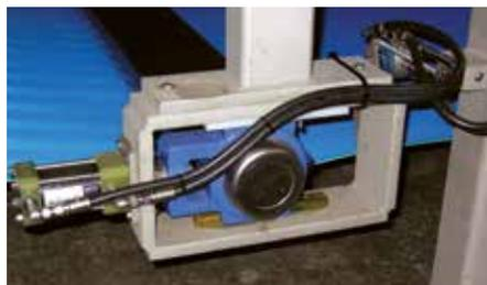
**8 Belt Tracking:** Tracking systems are available in both pneumatic and hydraulic systems providing trouble free operation. Tracking systems offer smooth and continuous tracking without excessive movement.
