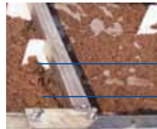
Significantly thickened slurry coming over Foil Doctor Plow.
