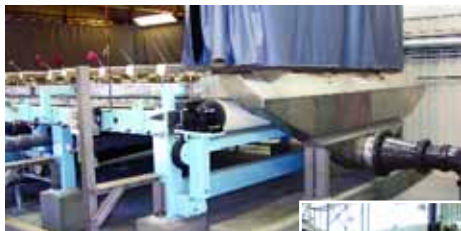
ABOVE: Industry first 4 meter wide Gravity Belt Thickener, 1200 gpm, City of San Francisco.
